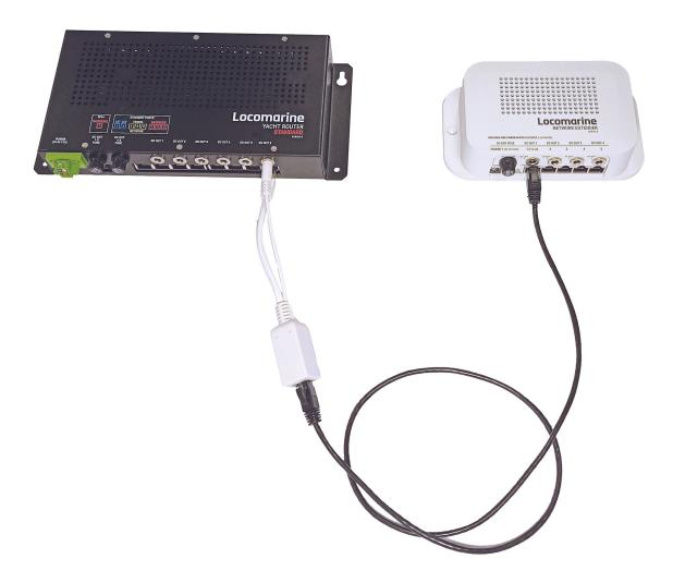
On a following photo you can see how to connect multiple Network Extenders to Yacht Router Standard (or any other Yacht Router model) using PoE injectors (supplied with a package) and Ethernet cables. Ethernet cable on a second Network Extender is is connected to first port (PoE). Please note that DC Out Ports on second Network Extenders will not provide DC power.
