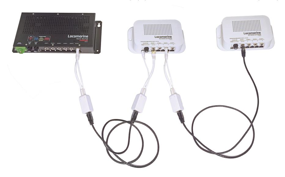
On a following photo you can see how to connect Network Extender to Yacht Router Standard (or any other Yacht Router model) using AC/DC power supply (supplied with a package) and Ethernet cable. DC Out ports on Network Extenders will provide DC power.
